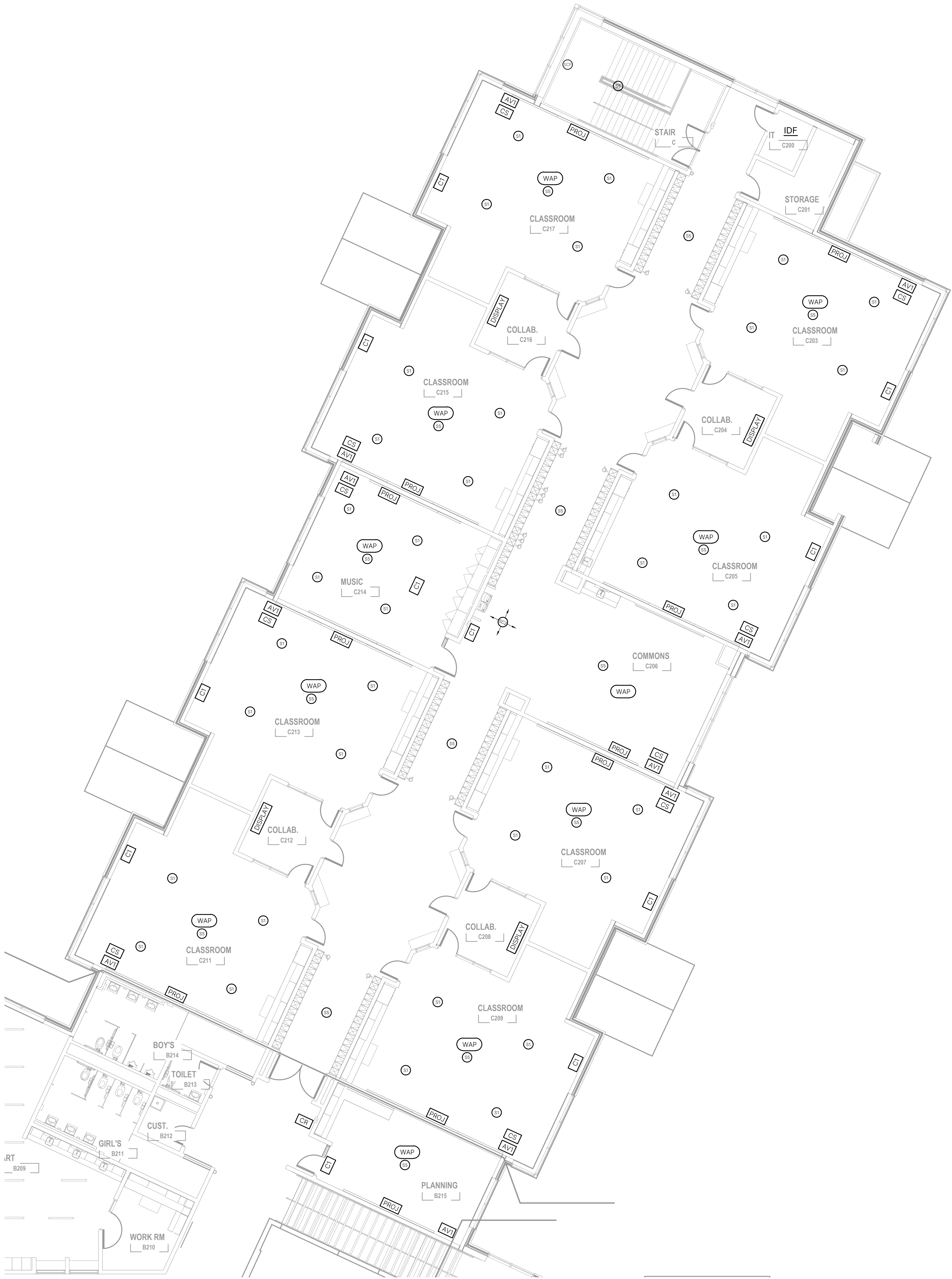
1/8" = 1'-0" SECOND FLOOR COMMUNICATIONS PLAN - ZONE 'C'
