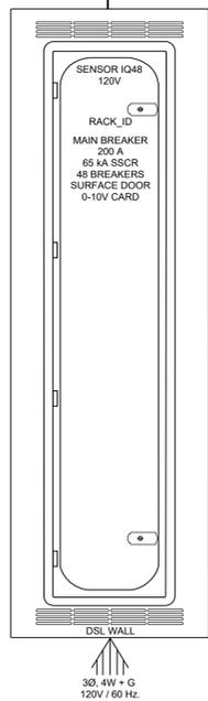
NOTE: ENCLOSURE MOUNT AND LINE VOLTAGE TERMINATIONS BY EC. SPECIFIED CABLE AND CONDUIT AS PER CODE BY EC. DATA TERMINATIONS AND PROGRAMMING BY TLV.
