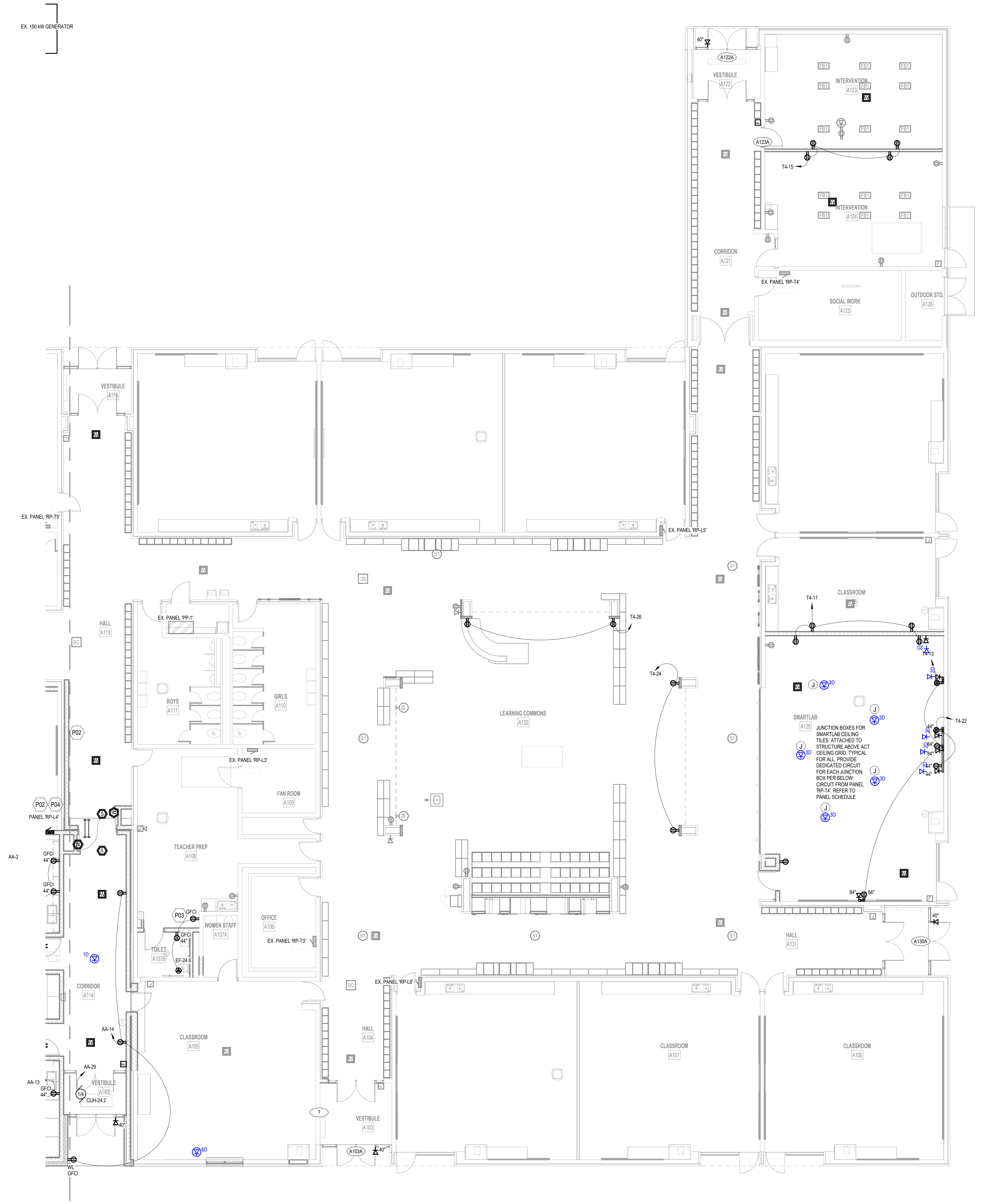
UNIT 'A' FIRST FLOOR POWER & COMMUNICATIONS PLAN 1/8" = 1'-0"
